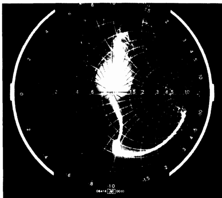
Fig. 10.34 Phase jumping of TDRO (reference [27], ©1984 Microwaves & RF)
